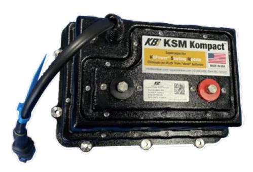
The Kold-Ban International (KBi) KSM Kompact<sup>™</sup>module provides an engine with the power it needs to start, even with a "dead" or rundown battery, then fully recharges in about 30 seconds. Designed for recreational boats and smaller commercial watercraft, the maintenance-free KSM Kompact stores the power until it is needed for up to several months. It can be installed in any orientation. https://koldban.com/ksm-kompact/.
