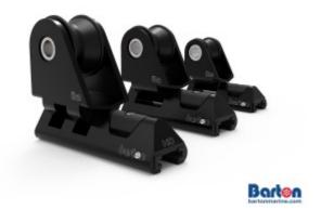
The new Barton sleek GT and HD Genoa Car range offers pin down and towable Genoa Cars in Spectro or black anodising, running on both 32mm and 25mm T Section track. Manufactured in the UK in high grade aluminium, the cars incorporate moulded nylon inserts to provide smooth free running precision, aluminium bearings and machined Ertalyte sheaves with a riveted tube axle for extra strength and to minimise friction on the bearings. Stainless steel plunger knobs
